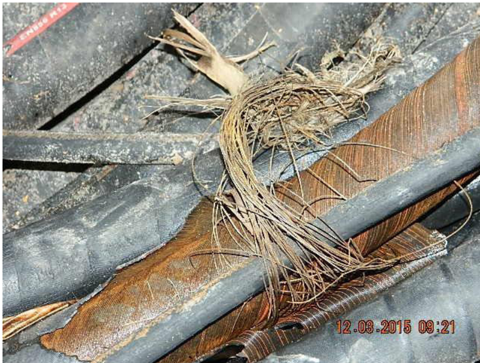
Metal hose braiding badly frayed, rendering the hose unsuitable for use
