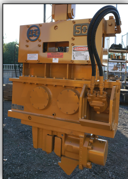
Model 50E with a standard 50 Clamp and single/double jaws
