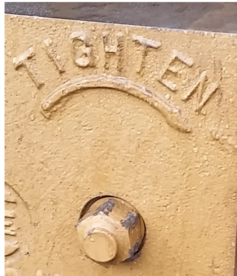
Caisson TIGHTEN label appears on one side of the clamp above the wedge screws.
