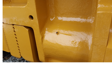
Grease-zerks are on the clamp cylinder near the jaws.
