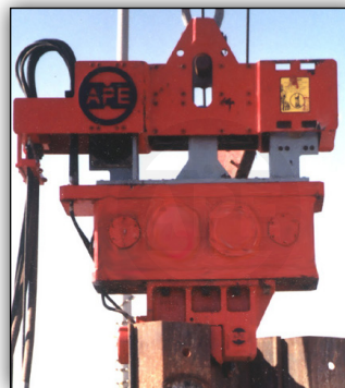
Model 150T Vibro with a Model 150 Clamp.
