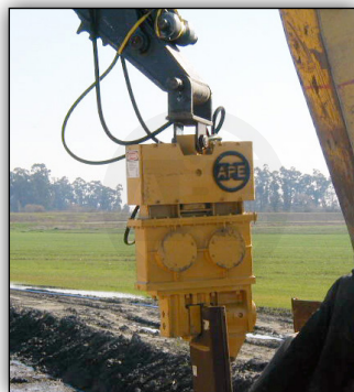
Model 20 Vibro with a Model 20 clamp.
