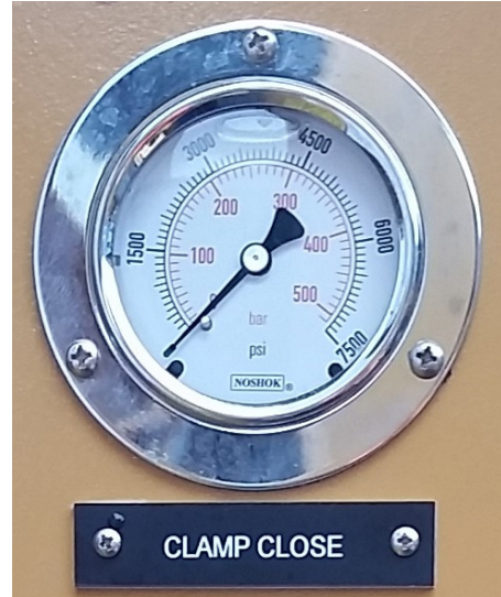
Power unit clamp CLOSE dial as seen beside the power unit control panel. Pressure measured in psi and bar.
