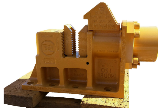
150 Sheet clamp painted for storage. The machined surface on the bottom will still require protection
